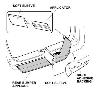
Remove the small right adhesive backing. Using the soft sleeve, firmly press the rear bumper applique against the rear bumper.
